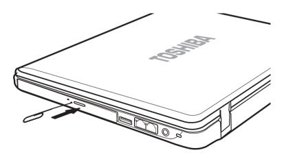
Manual release with the eject hole
